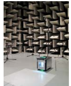
ISO 3744 acoustic test
