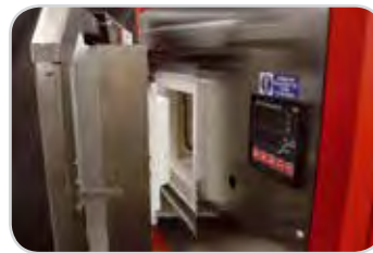
HtIndustry controller with 30 programs of 15 steps each
