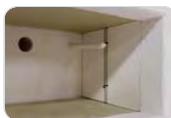
Thermocouple in furnace chamber and ventilation chimney
