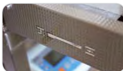
Sliding lever for controlling air supply
