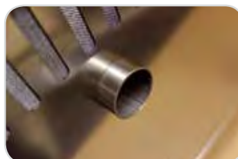
Chimney for the ventilation of the inner furnace chamber
