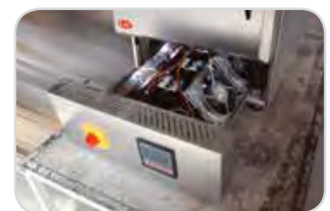
Pull out drawer with electro components for easy service access
