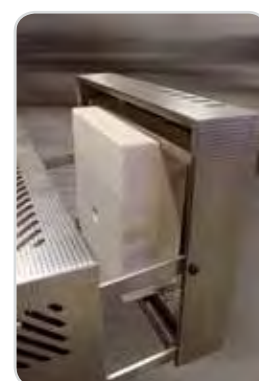
The door insulation with the peephole for batch control
