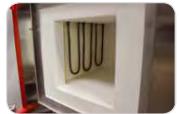
Exposed heating elements
