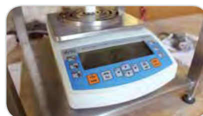
Digital scale placed under the furnace
