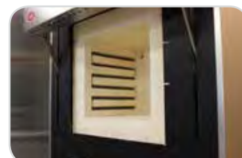
Heating coils in grooves built into the lining
