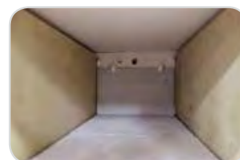
Furnace chamber with thermocouple and ventilation chimney
