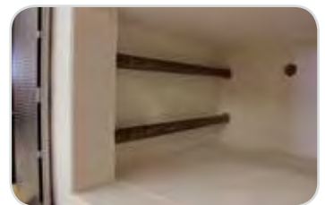
Heating elements in glass tubes
